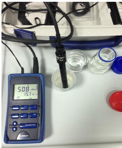
Figure 1. Determination of the EC with conductometric sensor
