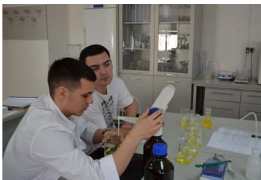
Figure 11. Determining the chlorine using the titrimetric evaluation
