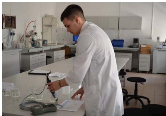
Figure 7. Laboratory measurements of pH, conductivity and dissolved oxygen
