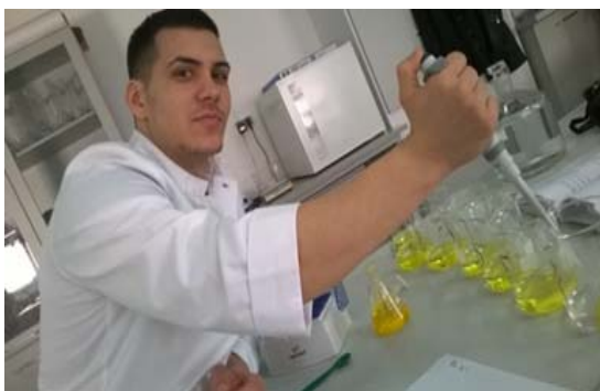
Figure 10. Determining the chlorine using the titrimetric evaluation
