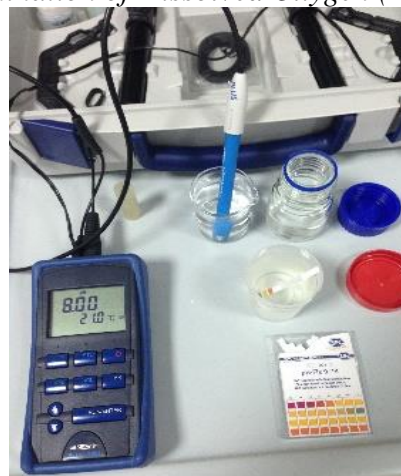
Figure 2. Determination of pH with pH sensor
