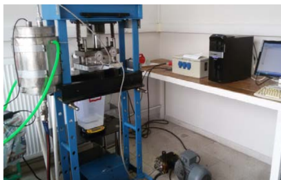
Figure 2. Cross flow flat sheet test unit in the lab scale
