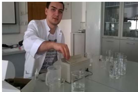
Figure 8. Determining the turbidity with a high precision stationary turbidity meter
