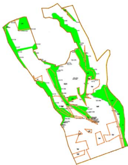
Figure 4. The differences between GPS and orthophotomap measurement on map – parcel 103/4 Green colour – forest land: GPS measurement, orange lines: orthophotomaps measurement (Source: own work, program C-GEO)
