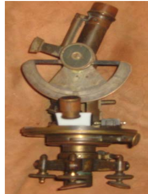
Figure 5. Theodolite Otto Fennel Sohne Kassel – 1920
