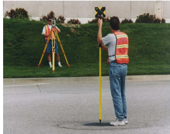
Figure 8. The measurement principle with reflector
