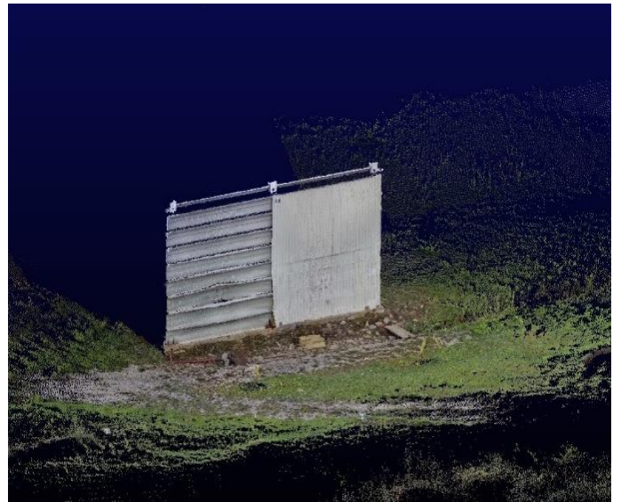
Figure 7. Uncleaned point cloud of the panels after the explosion
