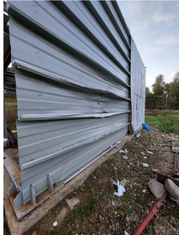
Figure 4. After-blast footage of the deformed panels
