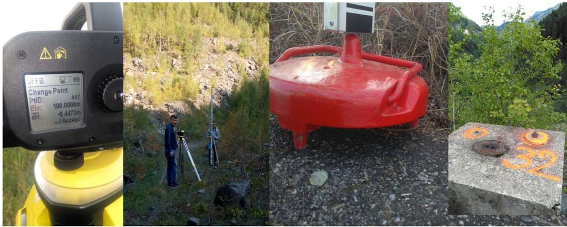
Figure 7. Progress measurements - Leica Sprinter 250M
