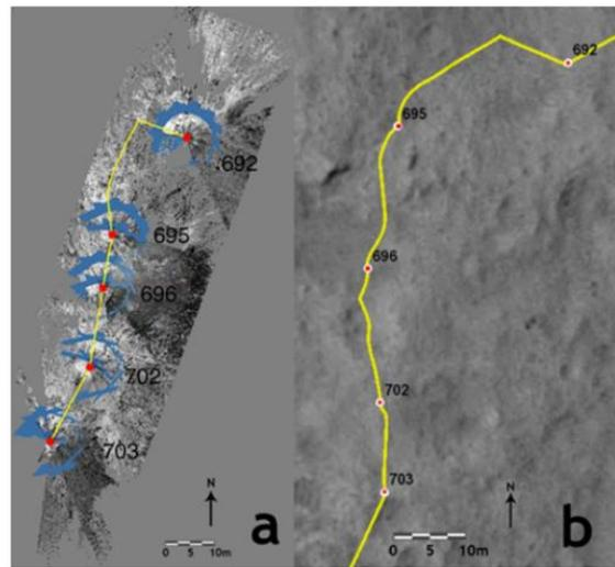
Figure 7. (a) Reconstructed traverse path (yellow) of Curiosity as determined using Agisoft Photoscan Professional and Navcam images from sols 692, 695, 696, 702, and 703. Red points show estimated rover position on these sols and blue polygons denote estimated camera poses. (b) Actual traverse map for Curiosity for sols 692-703.
