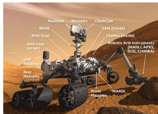
Figure 2. Instruments on board the Curiosity Rover
